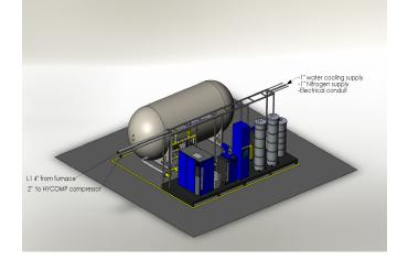
QuantumPure cryogenic recovery and purification system
